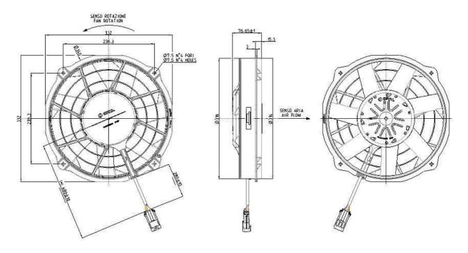
Fixing recommendation: use M6 bolts for fixing. Nominal tightening torque 5 +1/0 Nm Nominal torque defined for brand new, clean and lubricant-free bolts.
