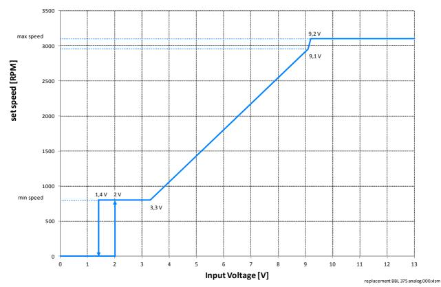
NOTE: tolerance on voltage threshold for minimum speed is 2 ±0.5 V
