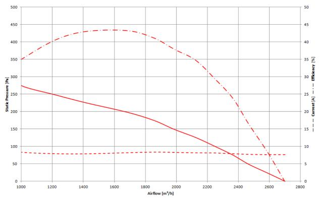
Air density 1.21 kg / m3 - Test number: #14048 – Test bench compliant to ANSI AMCA 210 TAMB = 20 % ± 5 % - UB = 26.0 V at the Drive connector
